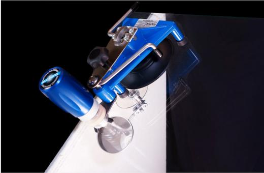
Screw the blue injector clockwise until it stops or the white seal dilates. You should see resin flowing into the impact. Hold this injector plunger position for around 5 minutes or until the impact is filled.
