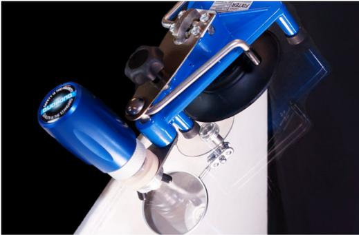
Screw the upper blue injector part clockwise until it stops. You should see resin flowing into the impact. Then hold this injector plunger position for 1 minute. You should see the white rubber seal expand.
