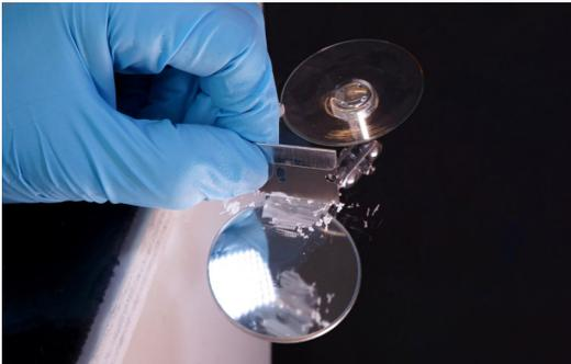
Remove any excess resin with a razor blade. Pull the razor blade over the repair area at a 90 ° angle and carefully scrape off the excess resin with an upward and downward movement.
