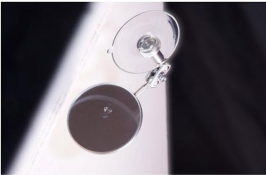
Apply a thin layer of gel to the suction cup of the inspection mirror and position the mirror under the repair area on the inside of the vehicle. The repair area should be clearly visible in the mirror.
