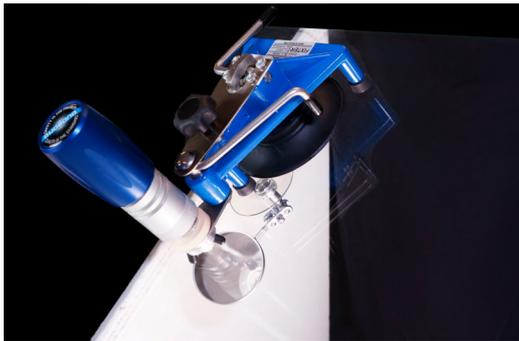
Turn the blue injector counter clockwise to create a vacuum. While doing this hold the silver part of the injector in place to avoid losing the seal to the glass.
