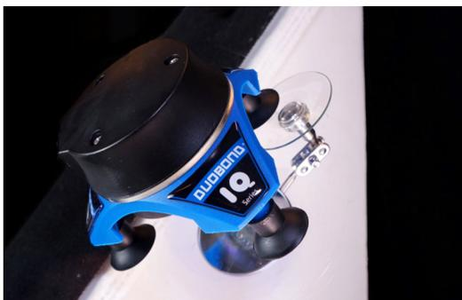
Place the UV lamp over the repair area, switch on the lamp and let the lamp automatically cure the resin and impact filler.
