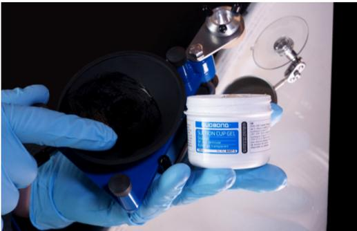
Apply a thin coating of gel to the suction cup of the Bridge.
