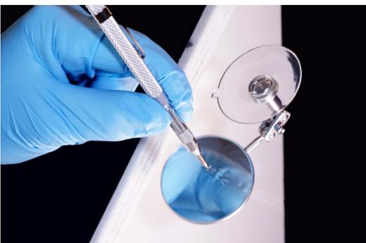
Clean the repair area from dirt and small glass splinters with a scratching pen.
