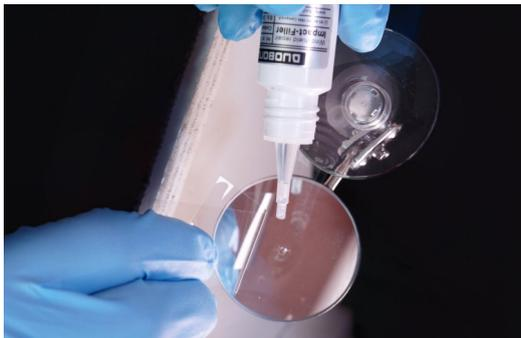
Apply a drop of Impact-Filler above the point of impact and let it run into the point of impact so that no air bubbles remain in the point of impact. Place the curing film over the damaged area.
