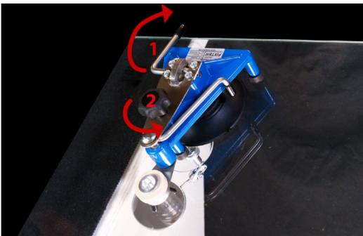
Press the suction cup firmly onto the glass and pull the handle (1) away from the sputnik head. (backwards) Lower the cup by turning the adjusting knob (2) clockwise.
