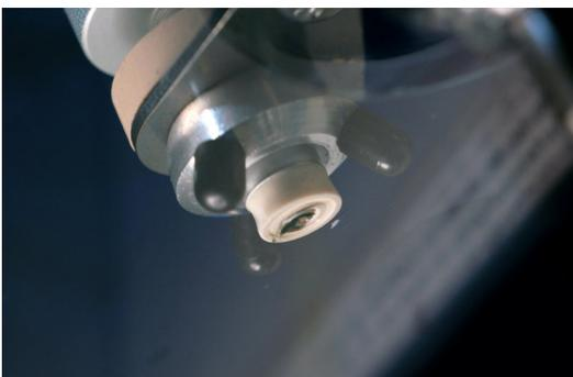
The dark ring of the injector, lying exactly around the point of impact, must be visible in the inspection mirror. Otherwise adjustment is necessary.
