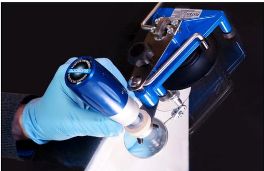
Screw the injector into the sputnik head. Turn the injector into the holder, and turn until the rubber of the injector gives a light print on the glass.
