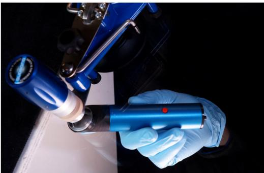
NOTE: The repair area can be gently heated using the Rezinator. Use the vibration function if air bubbles are still present. The Rezinator is designed to heat the impact point to a pre-determined level that should not cause any further damage or closing of cracks.
