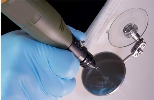
With small inaccessible impact points the impact area should be drilled using the carbide tipped drill bit.
