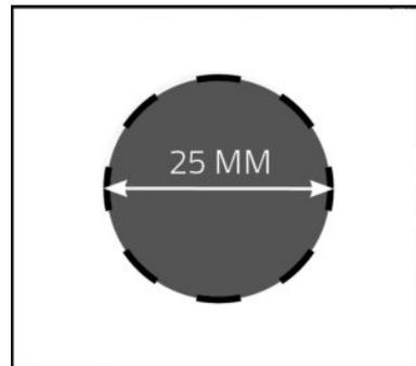
Do not repair damage greater than 25 mm (2 euro coin)
