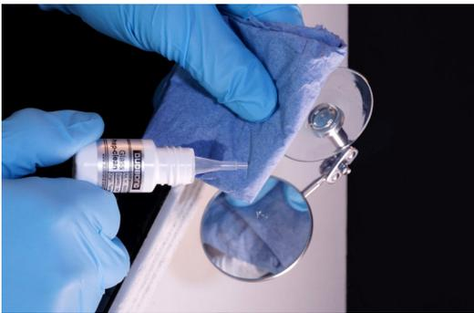
Use Duobond Prep-clean to clean the impact and remove any moisture. When applying Prep-Clean if the impact appears to reduce in size this indicates that there is access to the impact and drilling may not be necessary.
