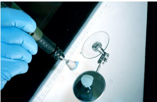
Clean the repair area with a lint-free cloth. Polish the surface with liquid polish and a Polisher on the drill until clear and smooth.
