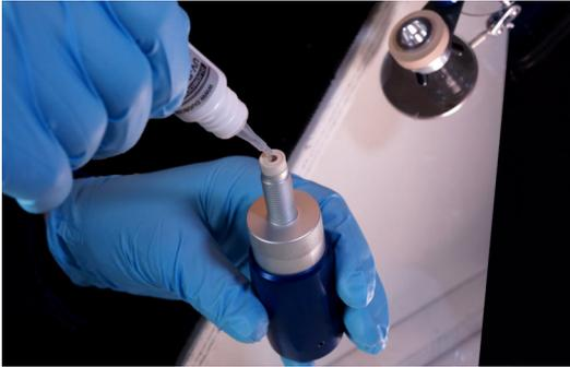
Invert the DART Blue unwind the blue cylinder 1/2 turn put 4 to 5 drops of resin in the injector cylinder and rewind a further 1/2 turn.
